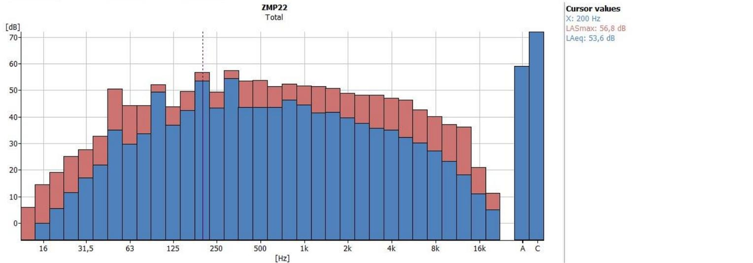
Figure 2-8: First LAI<sub>max</sub> value and LAS<sub>max</sub> average value at the measurement point ZMP22 (cursor position)
