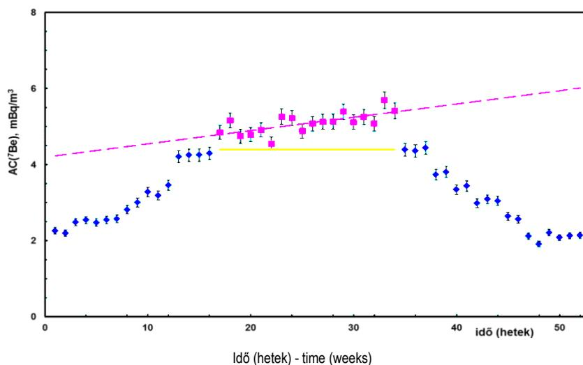
Figure 21.2.1-2: Change in time in the air activity concentration of  $^7\text{Be}$  in the environment of Paks Nuclear Power Plant.
