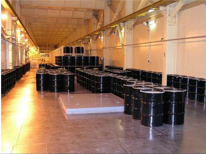
Figure 19.3.5-3: Temporary storage of solid radioactive wastes. [19-3]
