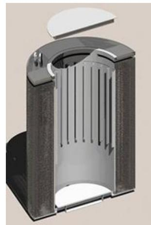
Figure 19.4.2-4: MAGNASTOR type storage cask and reinforced concrete structural shell. [19-34]
