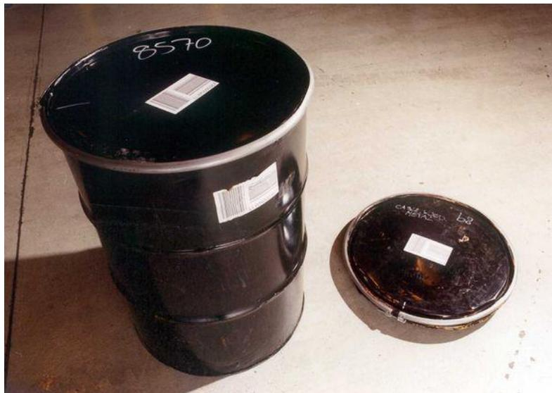
Figure 19.3.5-7: Low activity solid waste before and after supercompaction. [19-7]
