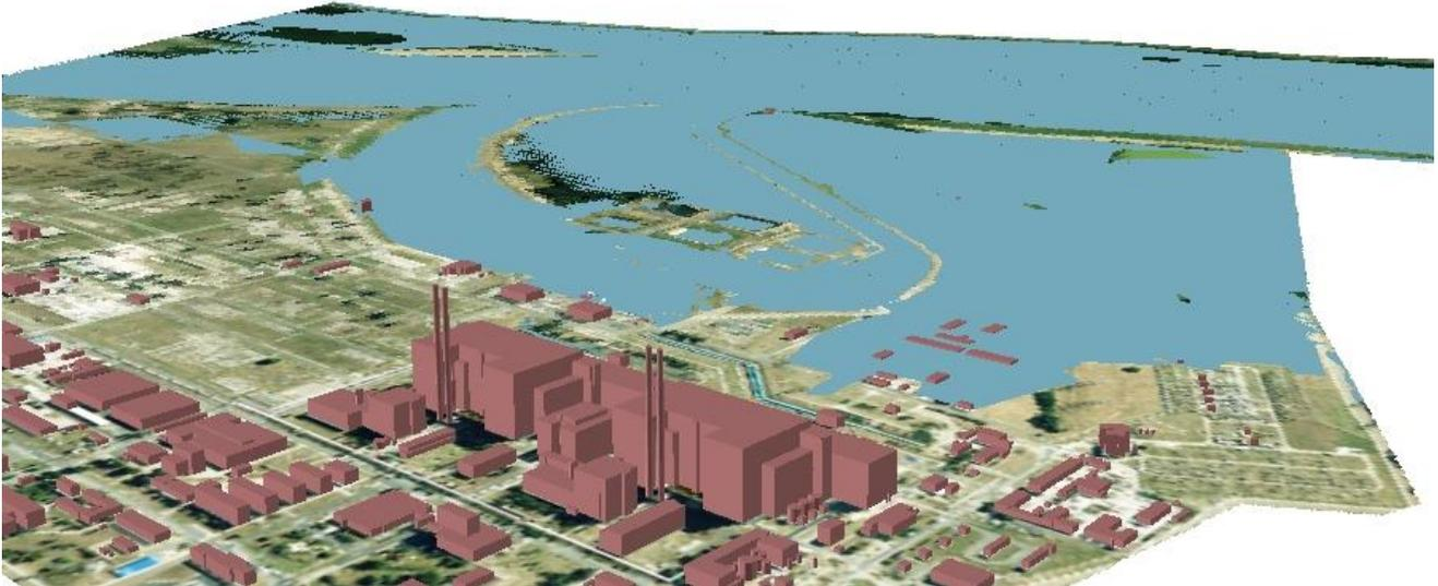
*Figure 11.9.1-10: Static inundation image developing when the Danube is at 96.90 metres above Baltic sea level*
